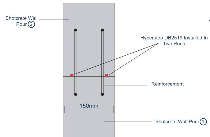
**NOTE:** The Joint Must Be Clean, Flat & Finished With A Trowel To Be Able To Accept Waterstop, Concrete Dags Must Be Removed By Others First.
