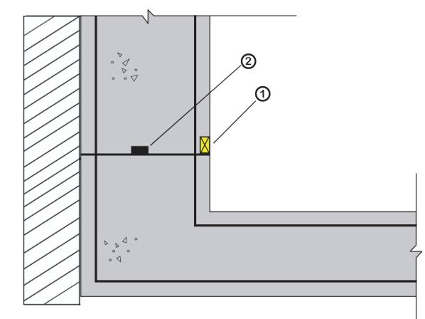
Formed rebate (1) approximately 25mm X 30mm, to be later filled with Bari-Cote waterproof grout.
