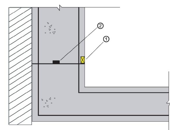
Formed rebate (1) approximately 25mm X 30mm, to be later filled with Bari-Cote waterproof grout.
